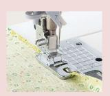
The spiral guide of this presser foot rolls the edge of the fabric to create a narrow rolled hem.
