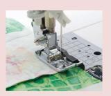
Always ensure needle is set to center straight stitch. Align the edge of the fabric with the presser foot guide to easily sew with a seam allowance of 1/4" (6.4 mm).
