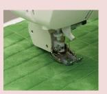
By inserting the quilt guide bar, this presser foot can be used to quilt equally spaced seams.
