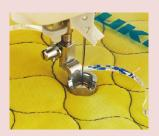
With a distance of 1/4" (6.5 mm) from the needle entry point to the outer edge of the presser foot, sew using a ruler as a guide. The front of the presser foot is lowered, making it easier to see the needle area. Adjust the height of the presser foot according to the thickness of the fabric.
