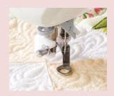
With the feed dogs lowered, you can freely move the fabric to draw using stitching.
