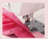
Change the stitch length, thread tension and presser foot pressure to adjust the amount of fabric that is gathered.
