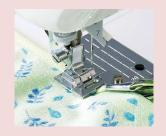
After tape with a width of about 0.75" to 1.0" (22 to 25 mm) is passed through the guide, this presser foot creates double-fold tape with a width of about 0.2" (5 mm) and sews it to bind the fabric. Single-fold tape with a width of about 0.4" to 0.5"(10 to 13 mm) can also be used.
