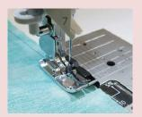
Always ensure needle is set to center straight stitch. Align the edge of the fabric with the presser foot guide to easily sew with a seam allowance of 7 mm.
