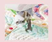
Use the screw to adjust the height of the presser foot according to the thickness of the fabric, so the fabric moves smoothly.
