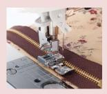
Since this presser foot has a pin on the left side and on the right side for attaching it to the presser foot holder, you can attach this presser foot on either side of the needle, depending on which side of the zipper is being sewn.
