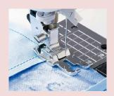
Always ensure needle is set to center straight stitch. Align the edge of the fabric with the outer presser foot guide for a seam allowance of 1/4" or with the inner presser foot guide for a seam allowance of 1/8". There are also marks at a 1/4" spacing at the front and back of the presser foot, allowing you to see the width of the seam allowance before and after needle entry.
