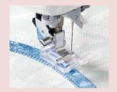
Since the front and back of this presser foot are short and transparent, appliqués and designs are easy to see, and you can easily sew sharp curves.
