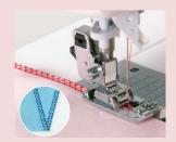
Sew with the edges of the fabric aligned with the guide. The prong in the opening of the presser foot presses down the edge of the fabric to prevent puckering. In addition, the amount of thread going into the stitching is adjusted by the thread crossing the prong, creating a clean finish with little shrinkage.
