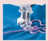
This presser foot has a hole for supplying cording to be sewn over. With the feed dog lowered, you can freely move the fabric to create simple embroidery with cording.
