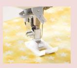
This presser foot, made of a fluorocarbon resin, smoothly feeds even vinyl-coated material and leather fabrics which may stick to a standard presser foot and are difficult to sew.
