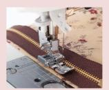
Since this presser foot has a pin on the left side and on the right side for attaching it to the presser foot holder, you can attach this presser foot on either side of the needle, depending on which side of the zipper is being sewn. This presser foot can cleanly sew along the edges of the zipper without hitting the teeth.
