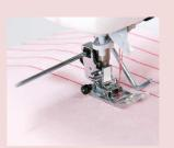
Insert this guide into the hole of the presser foot holder or the walking foot, and then sew while lightly tracing this guide along stitching.
