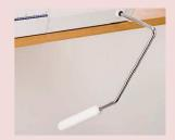
Using your knee to push the lever to the right raises the presser foot, and when you return it will lower the presser foot.
