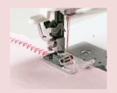
The groove along the bottom of this presser foot ensures that the presser foot does not catch on the stitching, so the fabric will be smoothly fed.
