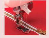
The position of the adjustable zipper presser foot can be changed over to the right and left of the needle to allow the sewing machine to sew the material while avoiding its thicker part such as a zipper.
